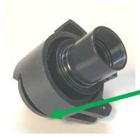
Push the eyepiece into the Eyepiece Adapter Cup so that the eyepiece is flush to the end of the cup and clamp into place so the eyepiece is secure.
