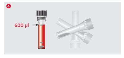
**4.** ... and mix the sample carefully by rotating 180 degrees.
