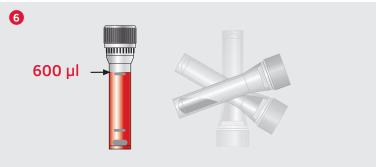
**6.** ... and mix the sample carefully by rotating 180 degrees.
