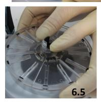
Do Not Pull Rotor Off The Spindle Clip Squeeze & Lift Vertically
